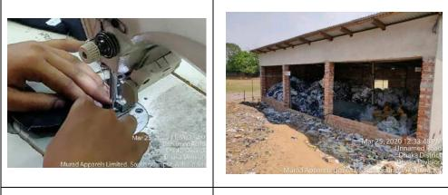
7. Approximately 30% sewing<br/>machines' eye guard, needle<br/>guard were found displaced.8. The wastage area was not found<br/>segregated as per the types and<br/>hazards.
