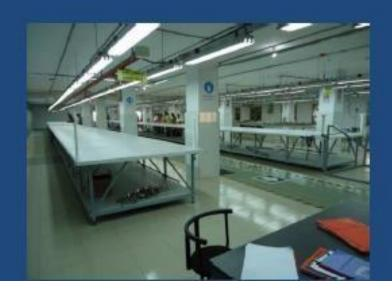
The pattern shapes for these garments maybe drawn on a paper marker placed on top of the lay, or information as to their shape and position maybe held within a computer, to be plotted similarly on the paper marker or used to drive an automatic cutter.
